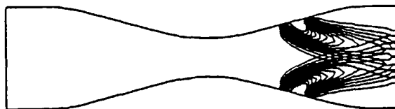
Figure 4 Solution of the system with N = 2 . Normalised number of droplets per unit volume contours of family 1 ( n_1/n_0 ), and family 2 ( n_2/n_0 ). ( N_{\min} = 0 , N_{\max} = 1.055 , \Delta n = 0.70 \times 10^{-1} )
